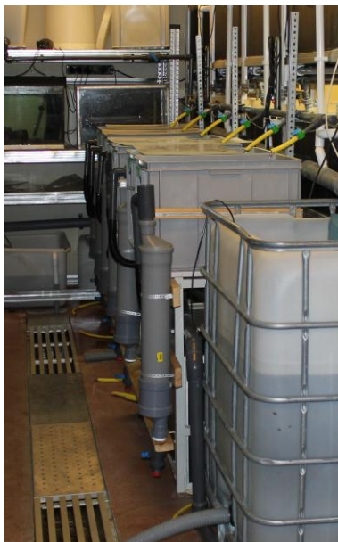
Figure 2. PVC tanks equipped with waste feed and faeces collectors. Foto. Aleksandar Vidakovic
