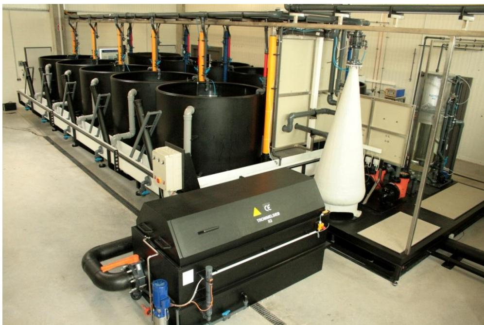
Figure 1. Recirculating aquaculture system which was used for the long-term study with turbot
